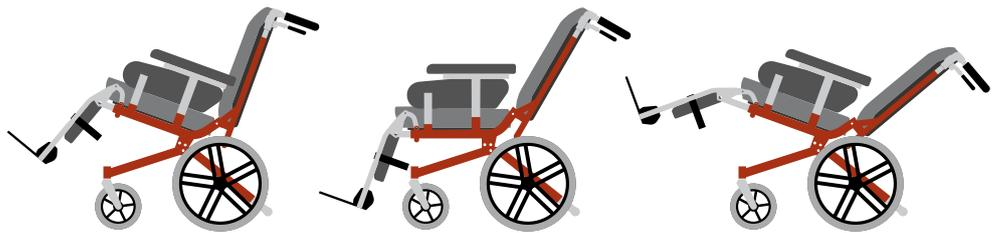
The seat unit can be tilted between 0° and +20° as standard. With an extended tipping bar the tilt can be increased to +30°. Extended tipping protection must be used. The back can be tilted steplessly using a gas spring from 0° to 30° as standard. With an extended gas spring the back tilt can be increased to 50°. Extended tipping protection must be used.
