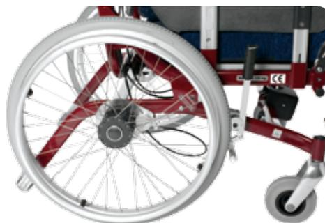
Seat height can be lowered - 5 cm on HD 500 model with alternative wheels 20" and 5" castors, enables the user to touch the floor with his or her feet.
