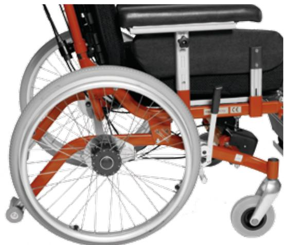
Seat height can be lowered -5 cm on the Bumblebee HD 500 model with alternative wheels 20" and 5" castors, enables the user to touch the floor with his or her feet.
