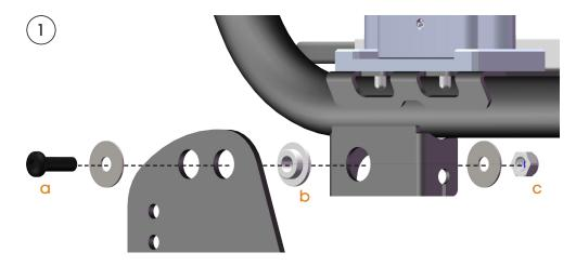
**Step 1**: See Figure . Remove the nut and washer (c) at the seat frame pivot point on each side. Leave the screws (a) in place to support the seating unit.
