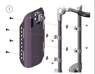
(2) Assemble the 4 back spacers between the backrest clamps and the backrest with the included bolts and nuts.
