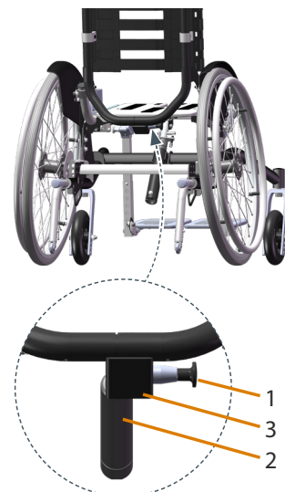
Figure 44. Locking pin for folding back rest
