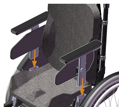
Figure 22. Armrests are inserted into the brackets on each side of the frame
