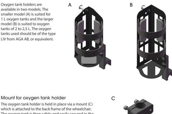
The oxygen tank is then safely and easily secured in the holder with two velcro straps.
