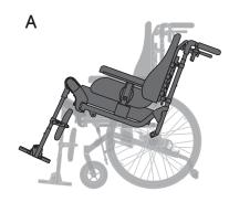
When there is a need backwards seat tilt can be increased to 0 to 30 degrees (B). This can, for example, be used if the user has need of a more backward tilted position for resting or for increased core stability. When backwards tilt is increased the drive wheels should be placed in the back position. See also the points under "Keep in mind" at the end of this document.
