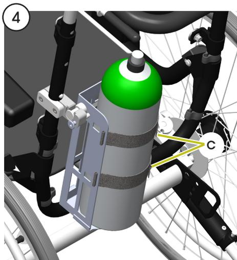
4. Place the oxygen tank in the holder and tighten the velcro straps (c). Make sure the straps are pulled tight so that the oxygen tank sits steady in the holder.
