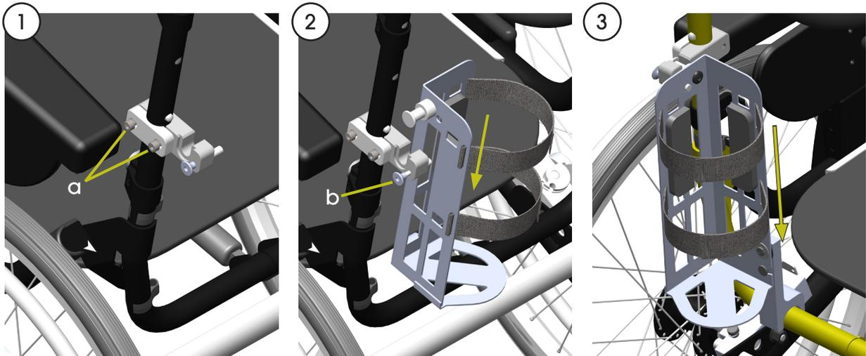
**NOTE:** The oxygen tank is not in the holder during assembly.
