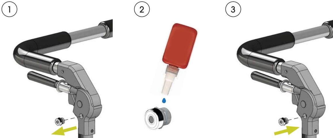
1. Remove the current release button from the push bar side unit.
