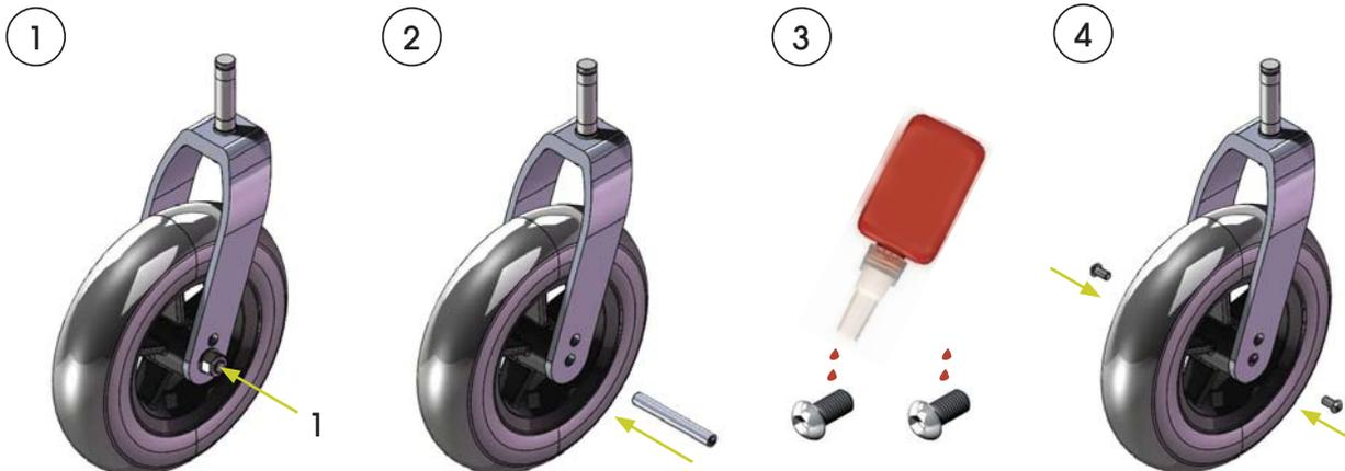
1. Disassemble the current bolt, nut, and washers (1) (The fork does not need to be removed from the wheelchair). These parts will not be re-used.
