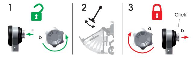
1 (a, b) Push and turn the knob counterclockwise. Now the knee joint is unlocked.
