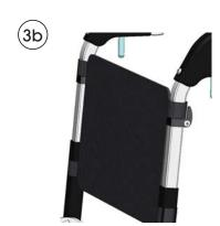
**3.** Finished! Adjustment of the height can be made by loosening the screws a little and then move the fastening along the tube. Tighten the screws afterwards.
