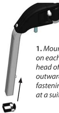
1. Mount one fastening on each tube with the head of the screw pointing outwards. Tighten the fastenings with the screws at a suitable height.
