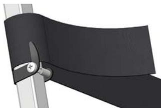
2. Mount the calf strap or the upper straps of the calf panel around the tube, above the fastenings. Fasten the straps on the backside with the velcro. When mounting the calf panel, also mount the lower straps around the tubes.
