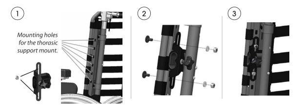
**1.** Position the mount so that the slots (a) correspond to two of the mounting holes on the backrest system. Make sure that the correct height for the support is achieved by choosing suitable holes.
