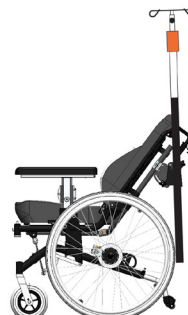
Diagram 10. A wheelchair with reclined backrest where the bracket has been rotated in order to keep the IV pole as vertical as possible.
