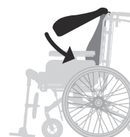
Diagram 12. Fastening straps around the Flexi-frame.
