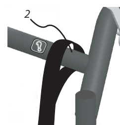
Diagram 51. Front tensioning during transport.
