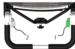
Diagram 14. Controls for the seat tilt (1) and recline functions (2).
