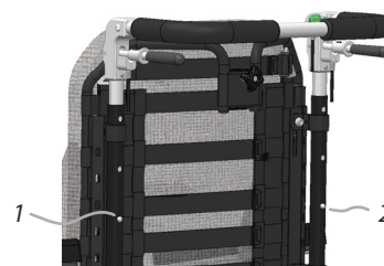
Diagram 11. The snap locks (push bar) alternatively the screws (separate operating handles) position.
