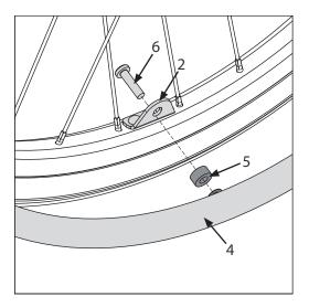
**1.** To move the hand rim (4) closer to the wheel, undo the four screws (1) and remove the hand rim.
