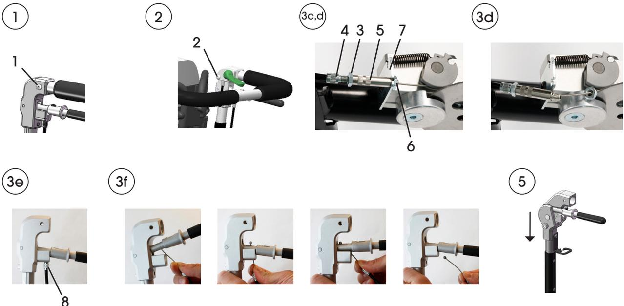
1. Remove the current push bar by loosen the screws (1) completely on both sides and pull it out.
